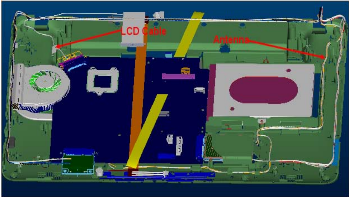
Figure 4-8-4 Remove the Wireless Antenna and LCD cable
